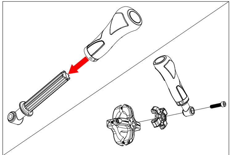
3. Adjust X-Clamp and Grip according to personal preference. Tighten M8-35mm Socket Head bolt to 12ft-lbs. Tighten M6 X-Clamp hardware to 4ft-lbs.
