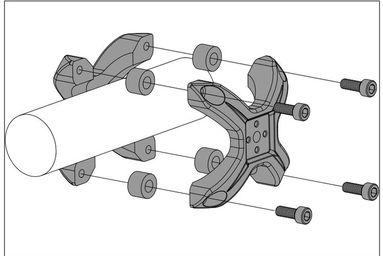
2. Slide Grip onto Grip Shaft. Using supplied M8 Bolt, loosely attach Grip Shaft and Base to X-Clamp.
